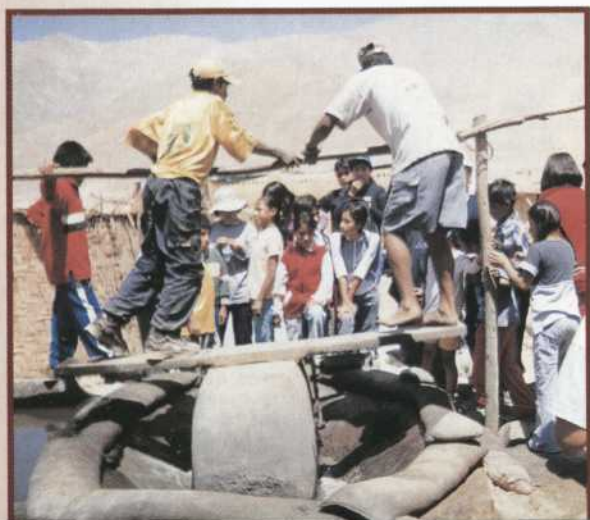
The Quimbaleta , a stone-grinding technique that dates back prior to the Inca culture. They pour water and mercury which causes the gold dust to clump together.
